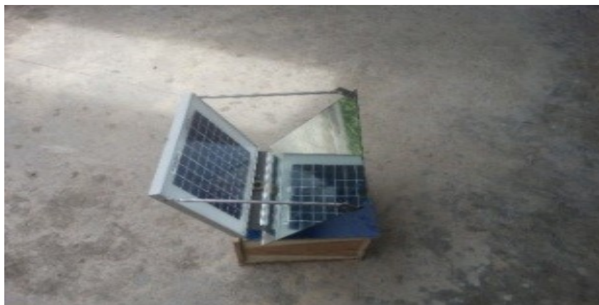
Figure 2 An instrumental set up of solar tracking system
