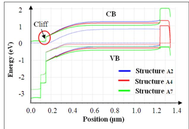
Fig. 4 The band diagram of some selected structures
