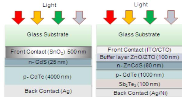
Fig. 1 Structures of the  $\text{CdTe}$  solar cells: (a) Conventional structure and (b) modified structure
